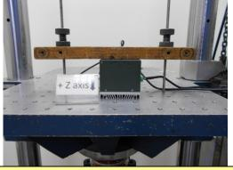
Mechanical Shock Test: +Z axis
