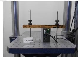
Mechanical Shock Test: -X axis
