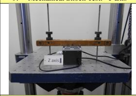
11. Mechanical Shock Test: -Z axis
