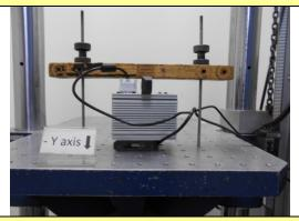
Mechanical Shock Test: -Y axis
