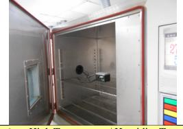
High Temperature/ Humidity Test 3. Low Temperature Test
