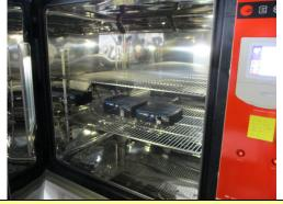
High Temperature/ Humidity Test; Low Temperature Test
