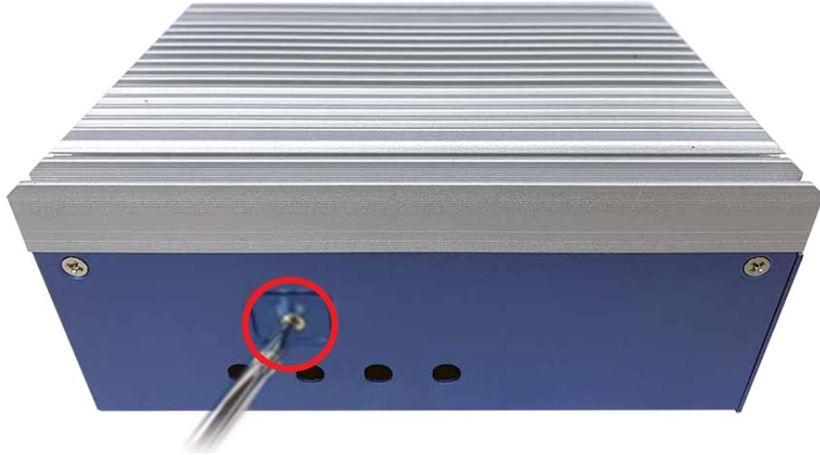
**Step 2** Install SIM card into to the SIM card slot and then close the SIM card cover.
