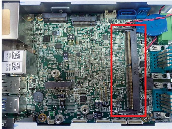
**Step 2** Install DDR4 RAM module into SO-DIMM socket.
